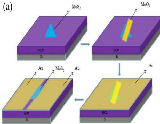
**Figure 3. (a)**  $\text{MoS}_2$  device preparation process.
