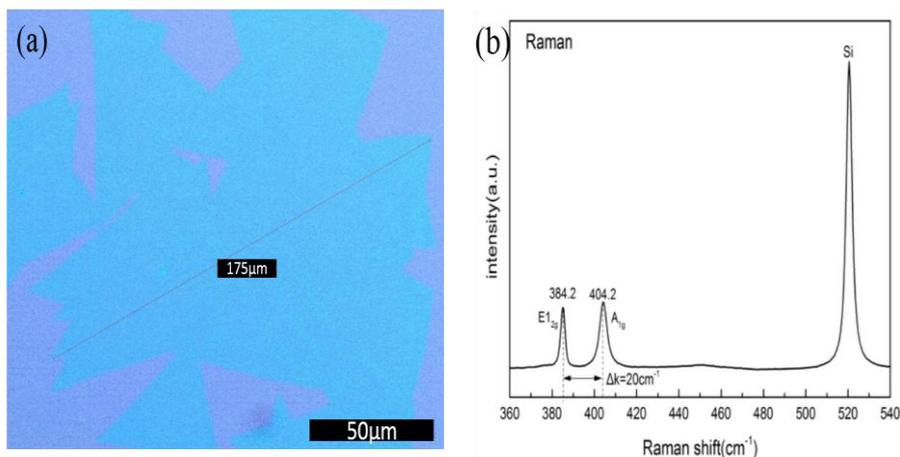
**Figure 1.** (a)Optical microscope images of  $\text{MoS}_2$ . (b) Raman spectra of multilayer  $\text{MoS}_2$ .
