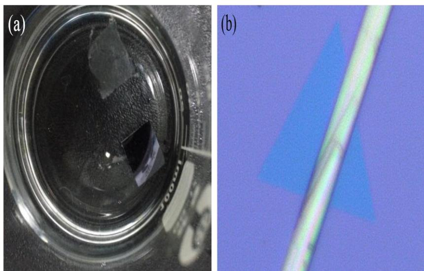
**Figure 2.**(a) The PMMA film was transferred. (b)  $\text{MoO}_3$  sheet for masking.
