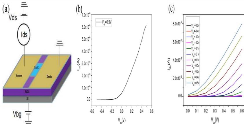
**Figure 4. (a)**  $\text{MoS}_2$  voltage measurement route. (b)  $\text{MoS}_2$  device transfer curve and output curve.
