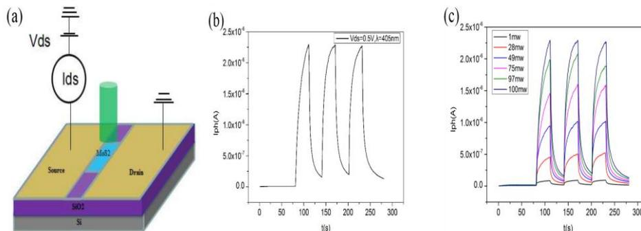
**Figure 5. (a)**  $\text{MoS}_2$  measurements from photo sensor. (b) Photocurrent of  $\text{MoS}_2$  at 405 nm wavelength. (c) The photocurrent of  $\text{MoS}_2$  at different powers at 405 nm wavelength.
